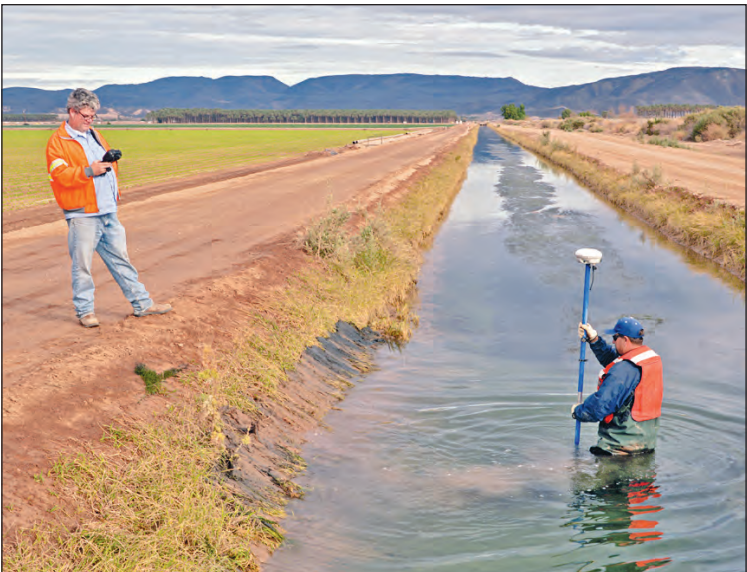
Pat Collon receives data from the GPS receiver on Roy's measuring stick to determine the exact bottom contour of an unlined canal. The survey crew performs measurements at regular intervals from edge of the roadway, at the point where the inclined bank becomes level and at the center of each canal, in order to determine a canal's actual volume.
