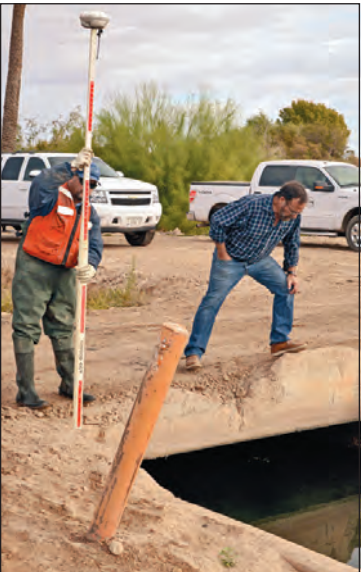
Ron Derma checks the flow of water as BOR Surveyor Roy Smith prepares his GPS equipped measuring stick to gauge the depth of a canal at the Mohave gates.
